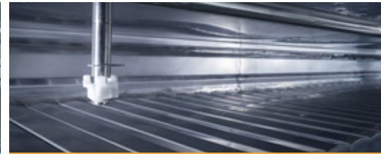
Clean-in-Place (CIP) Upgrade for Existing Freezers
